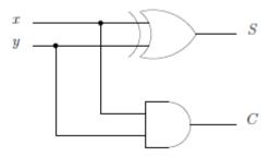
Figure 1. Half Adder Circuit
