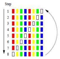
Figure 2: The sequence at which the LEDs turn on or off. The empty rectangles with black boarder represent and LED in the off state.
