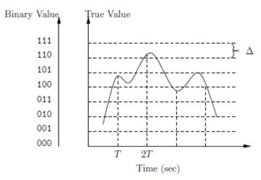
Figure 1. Sampling and Digitizing of a Continuous Signal
