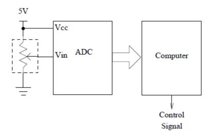
Figure 4. System Overview with the Variable Resistor that Represents the Variable Output of the Temperature sensor.
