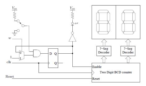
Figure 1: Circuit For Testing Your Reaction Speed
