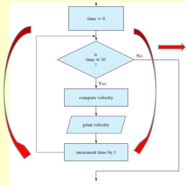
Figure 3.4 Flowchart for repetition structure.
