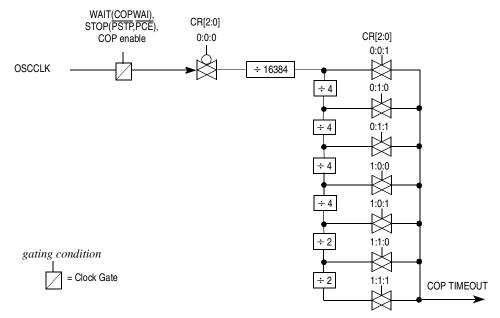
Figure 2. Clock Chain for RTI
