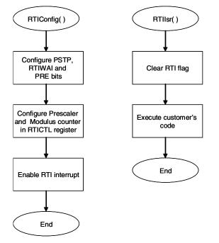
Figure 8. Configuring RTI and RTI Interrupt Service Function
