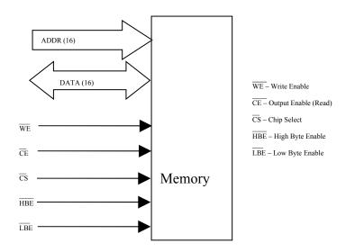
Need way to separate address and data Memory needs separate address and data busses
