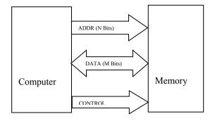
Computer with N bit address bus can access  $2^N$  bytes of data
