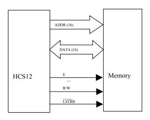
HCS12 has 16 bit address bus – can access 65536 bytes 1024 bytes = 1 kB 65536 bytes = 64 kB
