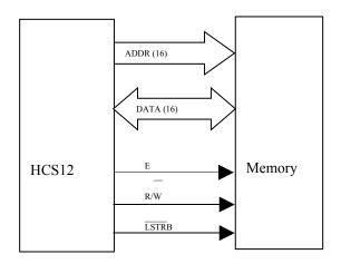
WRITE: a) HCS12 puts address on address bus and puts data on data bus
