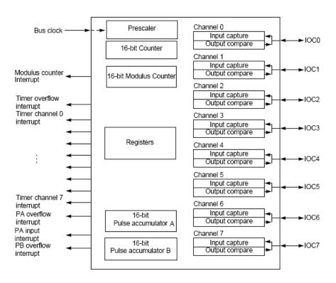
Figure 1-1 Timer Block Diagram
