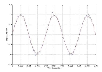
A sinusoidal signal with Gaussian noise embedded in it, and an averaged signal
