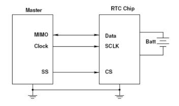
When used as a master in bidirectional mode, the Master Out Slave In pin becomes the Master In Master Out Pin.
