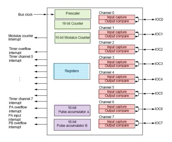
Figure 1-1 Timer Block Diagram
