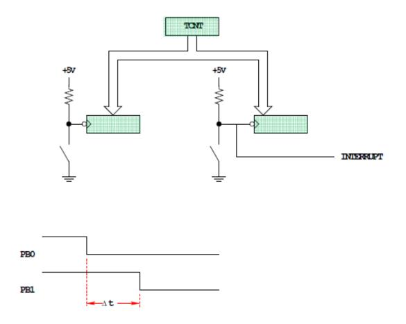
**Solution:** Latch TCNT on falling edge of signal
