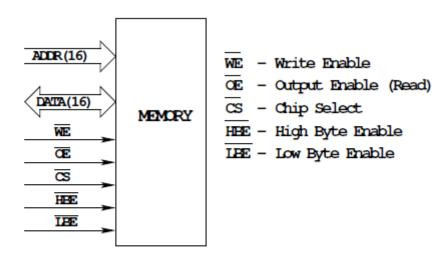
Memory needs separate address and data busses Need way to separate address and data
