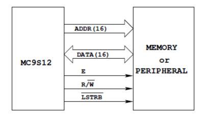
MC9S12 has 16 bit address bus – can access 65536 bytes 1024 bytes = 1 kB 65536 bytes = 64 kB
