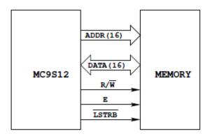
WRITE: MC9S12 puts address on address bus
