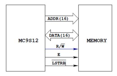
MC9S12 has 16-bit address and 16-bit data buses
