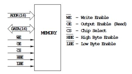
Memory needs separate address and data busses Need way to separate address and data
