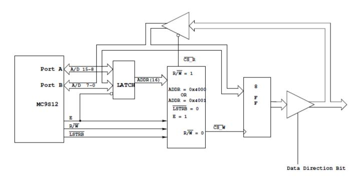
The data direction bit is the output of a flip-flop which was written to at another address of the HC12 For example, it could be Bit 4 of address 0x4002
