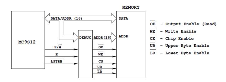
MCS12 has 16-bit address and 16-bit data buses Requires 35 bits
