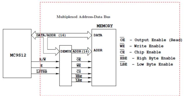
MC9S12 has 16-bit address and 16-bit data buses
