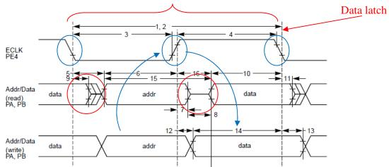
Table A-20 Expanded Bus Timing Characteristics
