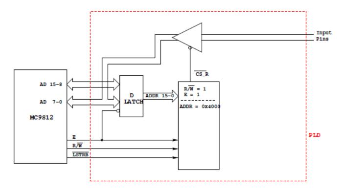
Reading from address 0x4000 (ADDR = 0x4000, R/W high, E high) will bring CS\_R low This will drive the data from the input pins onto the data bus The MC9S12 will read the data on the input pins on the high-to-low transition of the E-clock
