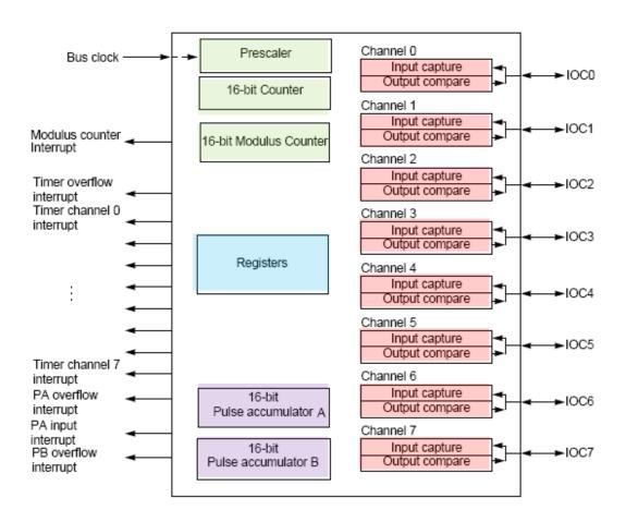
Figure 1-1 Timer Block Diagram
