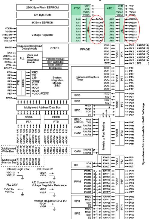
Figure 1-1 MC9S12DT256 Block Diagram
