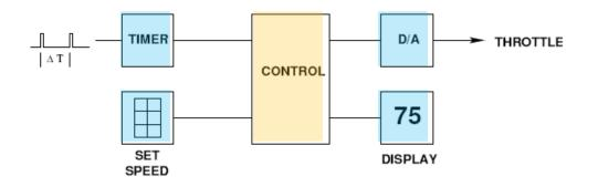
$\Delta T$  = time for one revolution of wheel. **Speed** = C/ $\Delta T$ , where C is the circumference of the wheel
