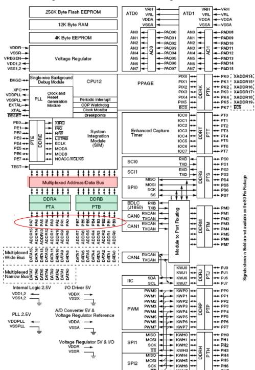
Figure 1-1 MC9S12DT256 Block Diagram
