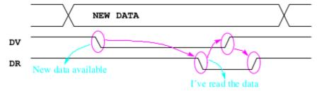
Use two lines — Handshake — sender knows when receiver is ready for new data.
