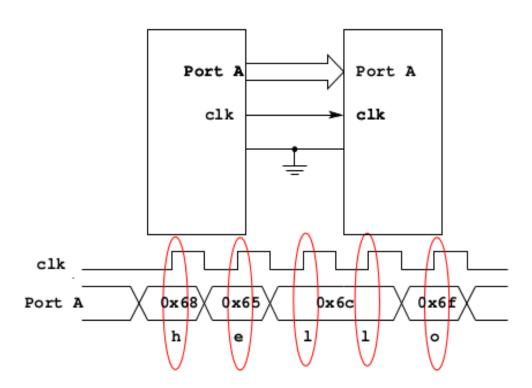
Need 10 wires to transmit 8 bits of data
