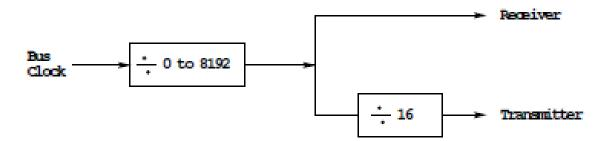
• With a 24 MHz bus clock, the following values give typically used baud rates.
