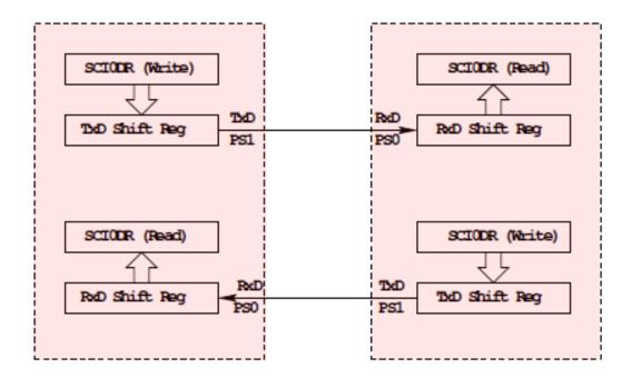
SCIODR receive and transmit registers are separate registers. distributed into two 9-bit registers, SCIODRH and SCIODRL
