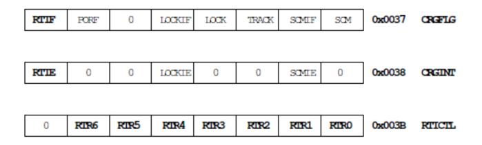
• To use the Real Time Interrupt, set the rate by writing to the RTR 6:4 and the RTR 3:0 bits of the RTICTL, and enable the interrupt by setting the RTIE bit of the CRGINT register
