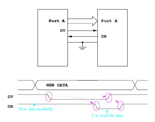
Use two lines — Handshake — sender knows when receiver is ready for new data.
