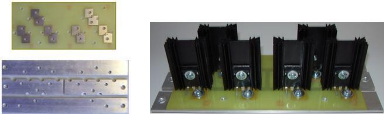
Figure 4. 2 : High Current MOSFET and Diode Layout
