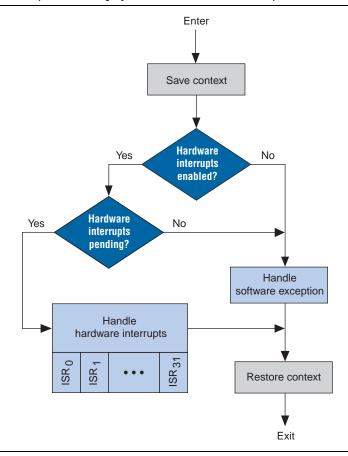
Figure 8-1. HAL Exception Handling System with the Internal Interrupt Controller
