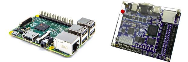
Figure 2. The Raspberry Pi 2 B, and Altera DE0 development boards.
