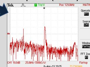
Figure 8: Amplified Noise Spectrum (0-250kHz)
