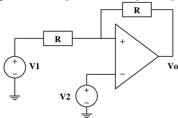
$$I = \frac{V_1 - V_2}{R}$$
