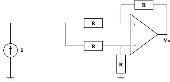
$$V_+ = \frac{V_I}{2} \quad I_- = I_+ = \frac{I}{2}$$
