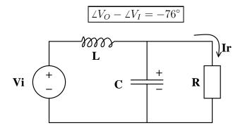
8. Derive the differential equation for  $i_R(t)$  in the standard form.
