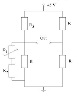
$R_S$  is the strain gauge. R should be slightly larger than  $R_S$  (perhaps  $121 \Omega$  if  $R_S = 120 \Omega$ ), and  $R_1$  and  $R_2$  should be much larger,  $10 k\Omega$  (for  $\pm 0.5\%$  adjustment range) or  $1 k\Omega$  (for  $\pm 5\%$  adjustment range). You may need to experiment by varying the values of the resistors R slightly to give you the adjustment range you need.
