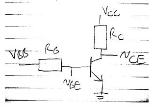
choosing  $R_B$  for a base current of 0.01 mA when  $V_{BB} = 10$  V. What do you expect  $I_C$  to be? Pick  $R_C$  to get  $V_{CE} = 5$  V when  $V_{CC} = 10$  V.
