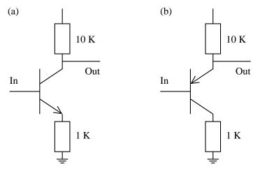
(a) For the common-emitter amplifier with emitter resistance we have
