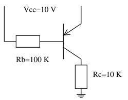
This transistor is clearly in cutoff mode, which means that  $I_C = I_B = I_E =$ , and then  $V_B = V_E = V_{CC} = 10$  V, and  $V_C = 0$  V.
