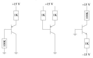
For the first circuit it is active mode because the bias cannot be at a lower voltage than the collector. We have  $V_C = 0$  V, and
