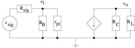
Including the signal generator and load resistor. Open-circuit gain  $A_{vo}$ :
