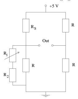
$R_S$  is the strain gauge. R should be slightly larger than  $R_S$  (perhaps  $121\,\Omega$  if  $R_S = 120\,\Omega$ ), and  $R_1$  and  $R_2$  should be much larger,  $10\,\mathrm{k}\Omega$  (for  $\pm 0.5\%$  adjustment range) or  $1\,\mathrm{k}\Omega$  (for  $\pm 5\%$  adjustment range). You may need to experiment by varying the values of the resistors R slightly to give you the adjustment range you need.
