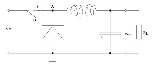
We will first plot the inductor current and voltage  $V_X$  for continuous operation. Here it is
