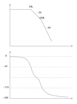
6. What is the closed loop gain corresponding to 45° phase margin? What happens if you make the closed loop gain smaller? larger? Design a inverting amplifier which has this phase margin.
