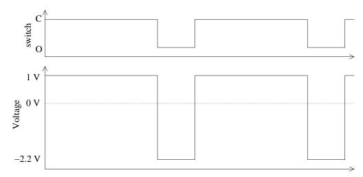
During discontinuous mode the closed-switch time is shorter, the time to discharge is the same, and the voltage across the inductor drops to zero at the end of the discharge period.
