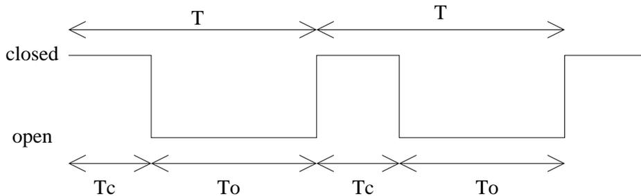
When the switch is closed the voltage  $V_{in}$  is applied across the the inductor, and the current through the inductor rises as function of time,  $t$ , since the start of the closed period.
