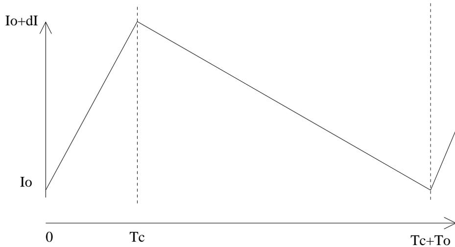
As you can see, there is always some current flowing greater than  $I_L(0)$ . Remember that the current can only flow in one direction. Because  $V_{\text{in}}$  is positive, and because there is a diode in the circuit, the current through the inductor can only flow in the positive direction towards ground. Even if the minimum current is zero, there is still a non-zero current flowing on average, because the time  $T_C$  is determined by the ratio of input and output voltages.
