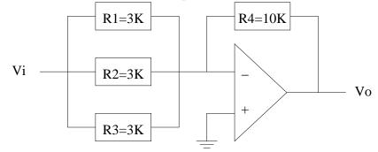
4. Compute the gain, noise, and signal-to-noise ratio with respect to each of the two inputs, for this circuit. How does SNR with respect to each input depend on the signal on the other input?
