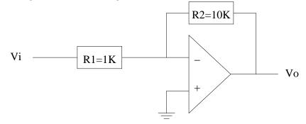
3. Compute the gain, noise, and signal-to-noise ratio for this circuit. Also compare the SNR of this circuit to the SNR of the previous circuit and discuss.
