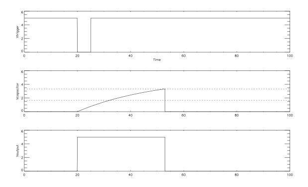
3. If  $R_a = 1 \,\mathrm{k}\Omega$  and  $C = 1 \,\mu\mathrm{F}$ , what is the duration of the pulse (assuming the triggering pulse is of even shorter duration)?
