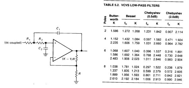
Here is where the mistake happened. We are going to assume that we can use a 4th order filter cascaded with a first order filter. This is not correct, but it is somewhat close. For the VCVS filter  $\omega_0 = \frac{1}{RC}$ , or
