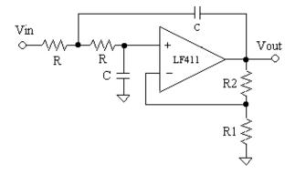
2. Build a second order Butterworth filter with 3-dB cutoff frequency of  $f_0 = 10 \,\mathrm{kHz}$ . Remember that if you attach the function generator directly to the input that either you should make R much larger than the output resistance of the function generator  $(50\,\Omega)$ , or you should include it in your calculation.
