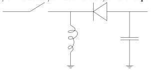
2. Derive an expression relating  $V_{\rm out}/V_{\rm in}$  to  $T_C$  and  $T_O$ , the switch closed and open time.
