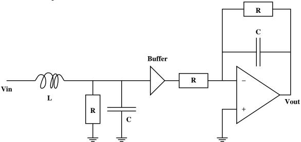
What goes into the non-inverting input is a second-order low-pass filter. The op-amp forms a integrator which is a first-order low-pass filter.
