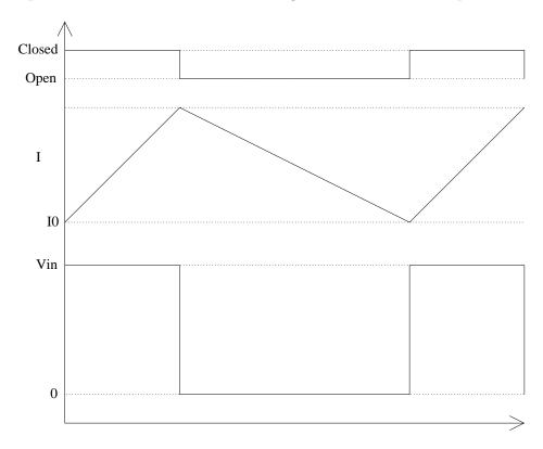
Next, we will plot the inductor current and voltage  $V_X$  for discontinuous operation. Here it is
