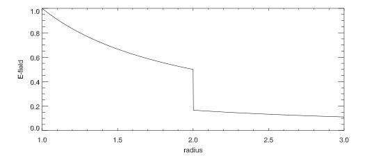
(g) If the purpose of the insulator is to reduce the maximum electric field, then placing the insulator at the center is best. If on the other hand the purpose of the insulator is to create the smallest electric field at the inside surface of the pipe it is better to place the insulator close to the pipe.
