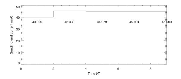
3. The final values for load voltage and current are those we expect from considering the transmission line a short,
