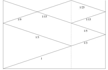
For the first  $4 \mu$ s the voltage is 1 V. For the next  $2 \mu$ s the voltage is  $1 + \frac{1}{3} + \frac{1}{9} V = 1.44 V$ . At  $6 \mu$ s the voltage jumps to  $1 + \frac{1}{3} + \frac{1}{9} + \frac{1}{15} + \frac{1}{45} V = 1.53 V$ , where the last term comes from the 1/3 reflection off the generator, but is not shown.
