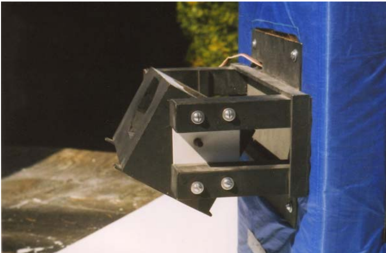
Axle side of scan platform - Note the bolts holding the plastic plate in place.
