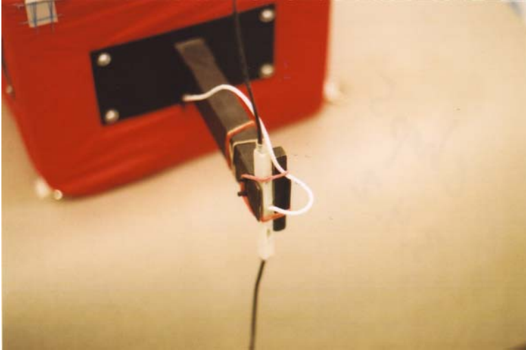
Business end of an antenna boom - An antenna is lightweight enough to be secured with a rubber band.
