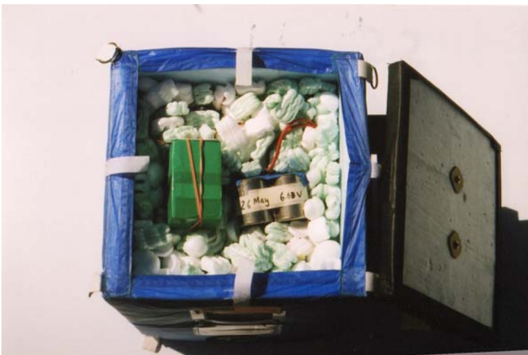
A Styrofoam-filled module - The packing peanuts keep components from bouncing around, especially during descent.
