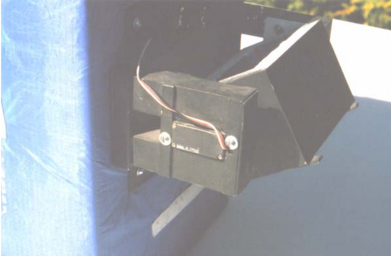
The servo side of a scan platform - The servo is bolted to popsicle sticks that have been epoxied to the scan platform booms.
