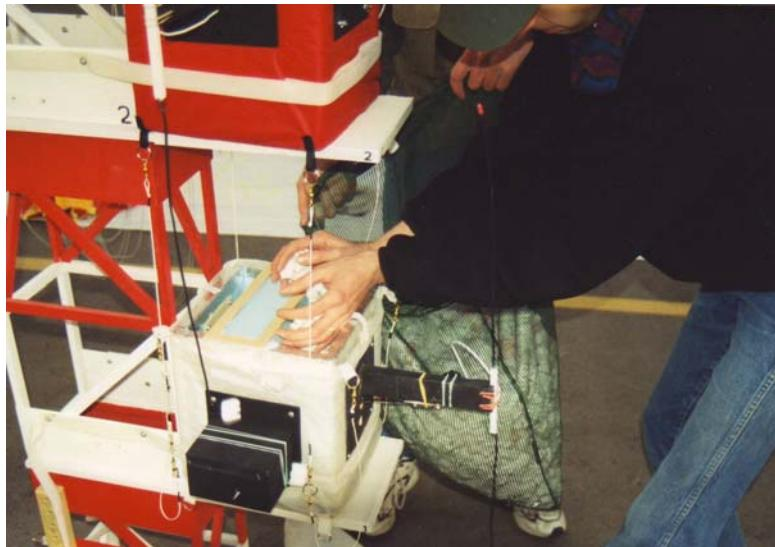
*Filling module with packing peanuts – Note the peanut bag*
