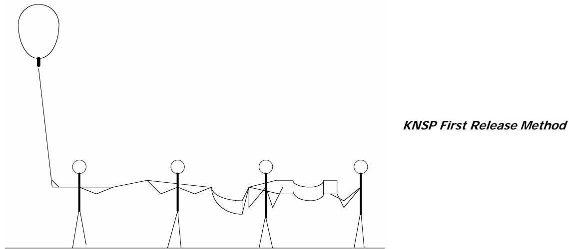
If there is any wind, the last handler must walk or run downwind with the module before releasing it. While running with the wind, let the module lift from your hands. When you do not run with the wind when releasing the last module, the stack swings like a pendulum below the balloon. This leads to all sorts of havoc should the module swing into the ground before gaining enough altitude to clear the ground or other obstacles.
