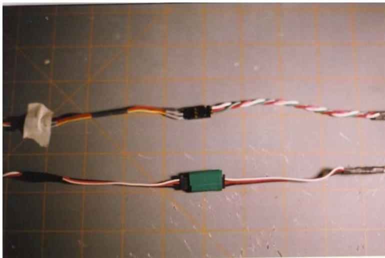
*Umbilical - Untaped example at top, properly taped umbilical on bottom*
