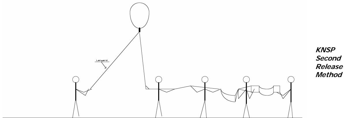
The first flight this method was used on, successfully launched the near spacecraft in higher winds that KNSP was accustomed to, however, one of the lanyards remained in front of the slow scan camera for most of the flight!
