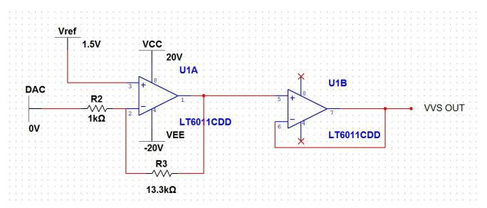
Assuming the DAC is running on a 1.5V Vref and running the output range of 3x Vref, or 4.5V (I looked this up in the TI datasheet for the microprocessor, the highest it should actually swing is 3.3V) we can achieve +/- 20V operation by using an inverting amplifier and we can use the extra opamp on the package as a follower.
