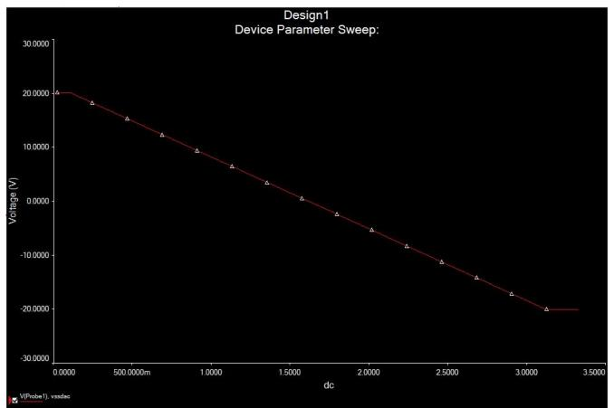
Differences in the opamp terminals are centered around 1.5v instead of ground to achieve bipolar operation. I figured an overshoot in the input would give us some breathing room to achieve the full range out of the DAC as it's recommended we have 256 steps, but with a 12bit DAC we get 4096.
