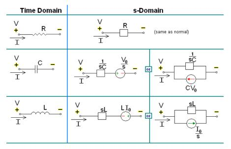
Note that the resistor is exactly the same in the time domain and the s-Domain. The sources are put in if there are initial conditions on the circuit elements. For example, if a capacitor has an initial voltage across it, or if the inductor has an initial current through it, the sources inserted in the s-Domain account for that.
