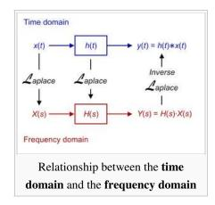
The transfer function is simply the Laplace transform of the impulse response:
