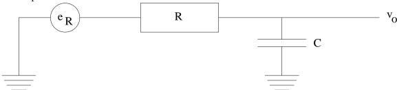
Now the resistor and capacitor form a RC low-pass filter with transfer function
